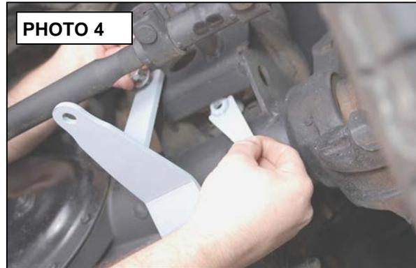
3. On drivers side secure with supplied  $\frac{1}{2}$ " &  $\frac{7}{16}$ " hardware .The supplied  $\frac{7}{16}$ " bolt / flag nut is used as shown in **Photo 4**. Repeat for Passenger side as shown in **Photo 5** and secure with supplied  $\frac{7}{16}$ " hardware for the stock mounting location and  $\frac{1}{2}$ " for the lower drilled hole.
