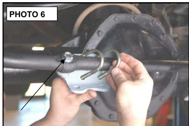
4. Locate and install the new center bracket as shown in **Photo 6** using the supplied  $\frac{1}{2}$ " bolt / hardware through the stock stabilizer mounting location and  $\frac{3}{8}$ " u-bolts on 02-07 models . **If the factory hole is not present in the tie rod the  $\frac{1}{2}$ " bolt will not be used. Make sure bracket is**
