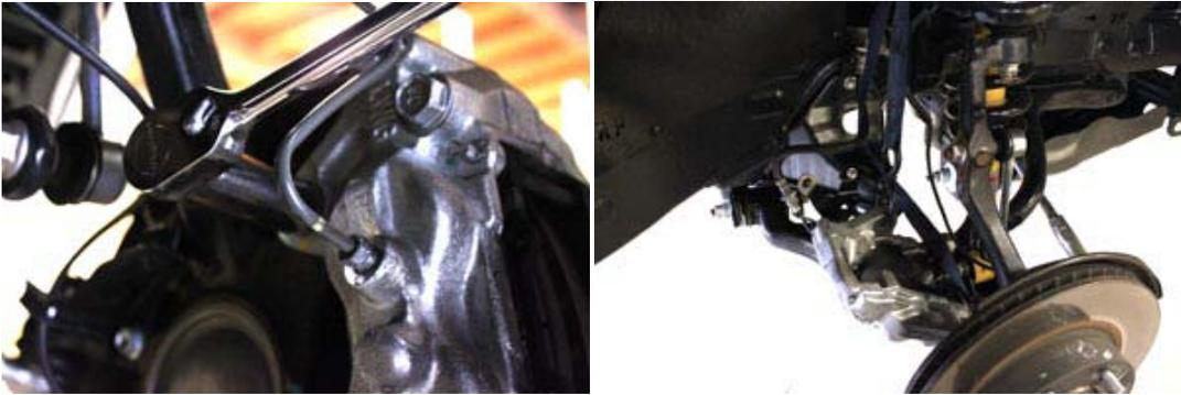
4. Remove brake rotor.
