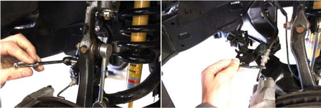
3. Remove brake caliper, then support it, do not allow it to hang from the brake hose.
