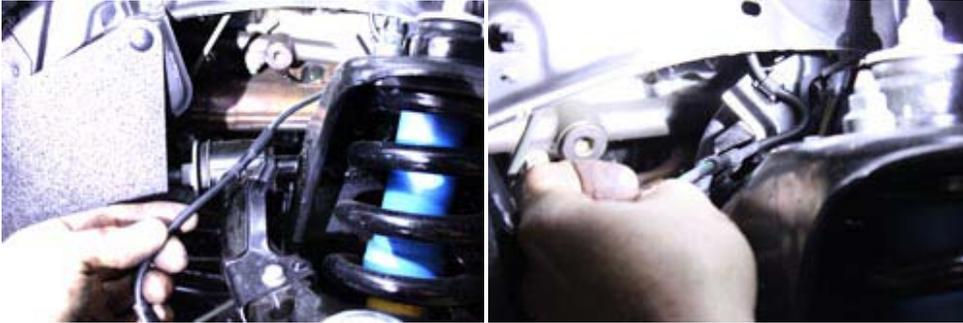
16. Remove bracket from upper control arm and discard, then remove ABS bracket from brake line bracket and discard
