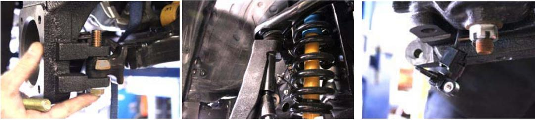
12. Attach lower ball joint / steering stop plate to the new spindle, tighten supplied 5/8"x3 1/4" bolts
