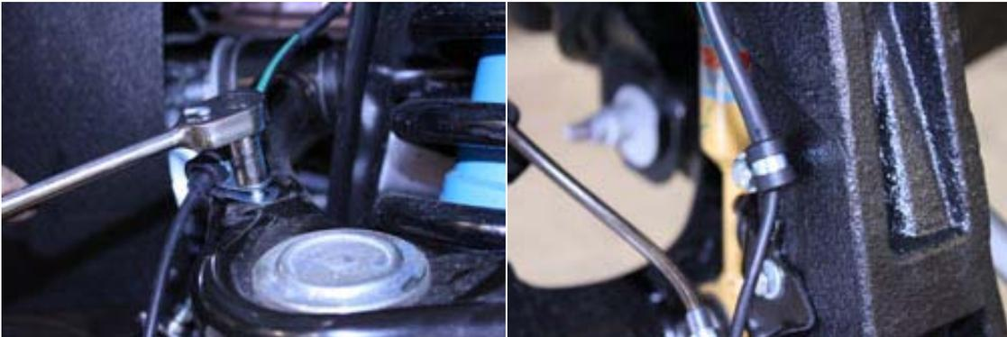
22. Tighten ABS sensor below the lower ball joint. Reinstall cotter pin to the upper ball joint and tie rod. See below for suggested brake line and ABS routing.
