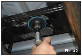
2. After cutting, flatten the area down with a grinding disc or roloc disc as pictured (Photo 2). Next, paint the area to avoid rust.
