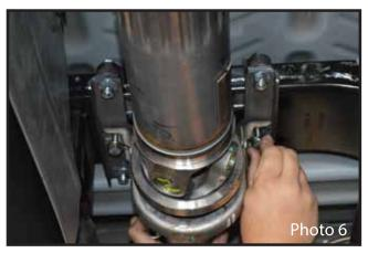
6. Bolt carrier bearing into place with the bolts going into the nuts on the angled bracket using the provided 3/8 bolts and washers. (Photo 6)
