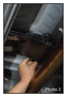
3. Slip the upper bracket in between the body of the truck and the carrier crossmember. Slide over to where the original carrier was mounted and align with the large hole in the frame. (Photo 3)
