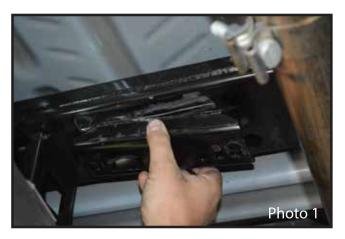
1. Remove the factory carrier bearing from the frame mount. Cut the OEM carrier mount off the frame using cut off disc. (Photo 1)
