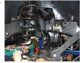
10. Unbolt the front radius rods using 21mm & 24mm sockets.
