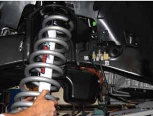
22. Install the bottom of the shock into the factory mount using the factory hardware. Tighten both ends of the shock hardware.
