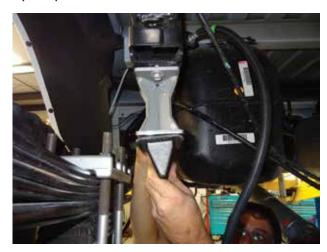
40. Install both of the rear McGaughy's shocks #3250. The shock shaft goes toward the top, upper mount and the main body goes towards the axle. Use the factory hardware from the stock shocks.
