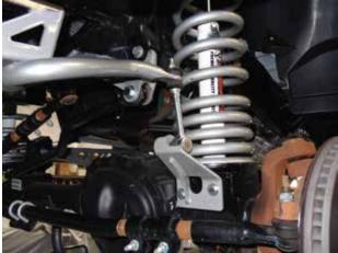
30. Put three U-clamps back on the stock drag link, using the stock hardware, & tighten.
