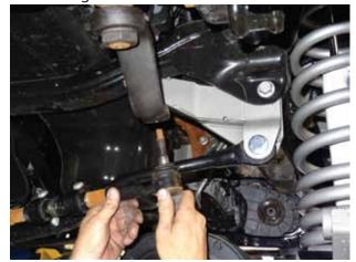
25. Install the new provided pitman arm onto the bottom of the steering box (where the stock one mounted) using the factory lock washer & nut.
