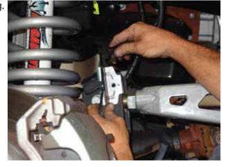
32.Re-install factory front drive-line. Put a small amount of lock-tite on each bolt before installing each bolt. Tighten to factory specifications.
