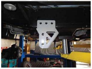
13. Now that the holes are drilled, remove the new bracket. The three holes, on the INSIDE only need to be drilled out (opened up) to 7/8". It is easiest to use a uni-bit (since it is shorter and easier to work around the stock exhaust) to drill the three holes. Do this on the driver and the passenger side inside three holes ONLY.
