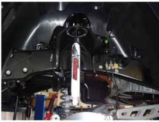
21. Install the new coil springs. The stock coil spring iscolator goes on top of the coil & it may be helpful to use a piece of tape to attach the iscolator to the coil so it stays while you are lifting the coil in. The progressive wound part of the coil goes towards the ground (the end where the windings are closer together).
