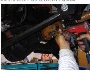
7. Use a 13mm socket and remove the stock brake line bracket from the driver side front axle and let the brake hose hang freely.
