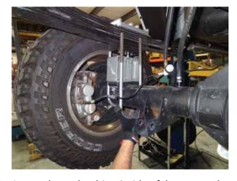
35. Lower down the driver's side of the rear-end so that you can install the new lift block between the leaf spring & the axle. The lift blocks are angled so the taller end of the block goes towards the rear of the truck.
