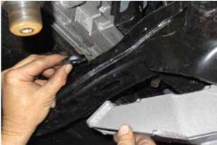
24. The bottom hole of the new track bar bracket is where the stock track bar bolts back up to the new 5/8" x 3 1/4" bolt with two washers & nylock nut that are all provided. Tighten all hardware.
