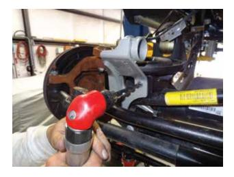
20. Install the new McGaughy's shocks using the factory hardware. Use a 9/16" x 3" bolt with two washers & a top lock nut to bolt the provided "clevis" bracket (black "U" bracket with 5/8" bolt welded on) around the new shock. The clevis goes on the end of the shock with the shaft, NOT the main body end. Install the upper end of the shock (the end with the clevis) to the factory shock mount hole. Use the provided 5/8" nut & tighten onto the welded on bolt on the clevis.
