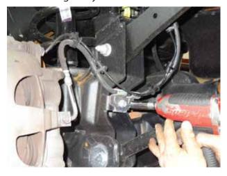
8. With a support still under the front differential, remove the front shocks.
