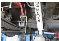
**10)** DON'T TIGHTEN LEAF SPRING OR SHACKLE BOLTS UNTIL THE VEHICLE IS ON THE GROUND IN ITS NORMAL STANCE.
