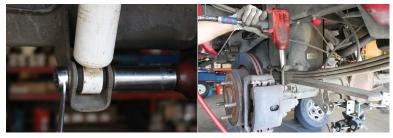
5) UNBOLT THE LEAF SPRING AT BOTH ENDS ALONG WITH THE SHACKLE & REMOVE.
