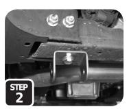
**STEP 2:** Loosely attach each of the two angled u-strap plates to the back of the rear cross member using the provided  $\frac{1}{2}$ -13 x 1  $\frac{1}{2}$ " bolts. *Note: ensure that the angled u-strap plates are angled outward.*
