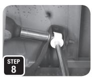
△ IF THE SHOCKS ARE MOUNTED UP-SIDE-DOWN, THEY WILL NOT WORK PROPERLY AND CAN GO BAD △
