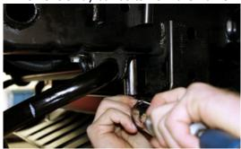
7. Install new Maxtrac Spacer, with bolt, nut, and washer. Install Rubber isolator.
